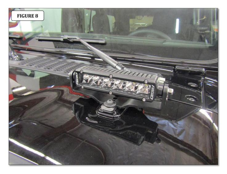
**Step-9** Repeat the above steps to install the light bracket and LED light assembly on the passenger side of the vehicle.
